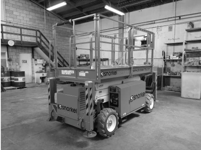
**Figure 10.1 - Correct Stowed Position**
