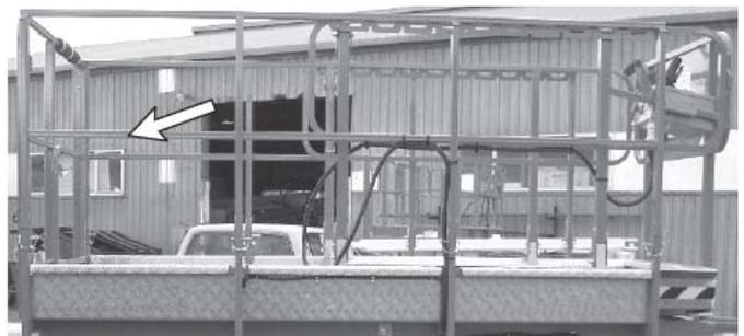
Figure 2.5 - Fall Restraint
