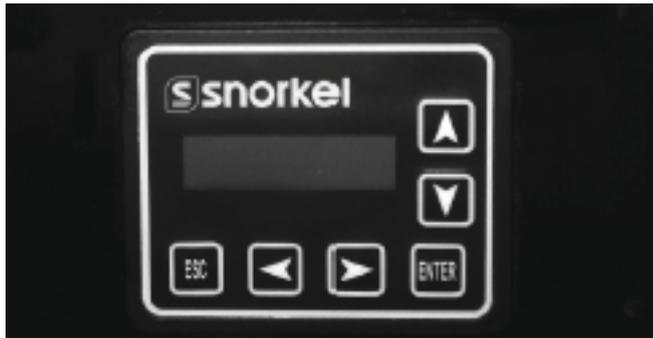
**Figure 4.1 - EzCal LCD Display**
