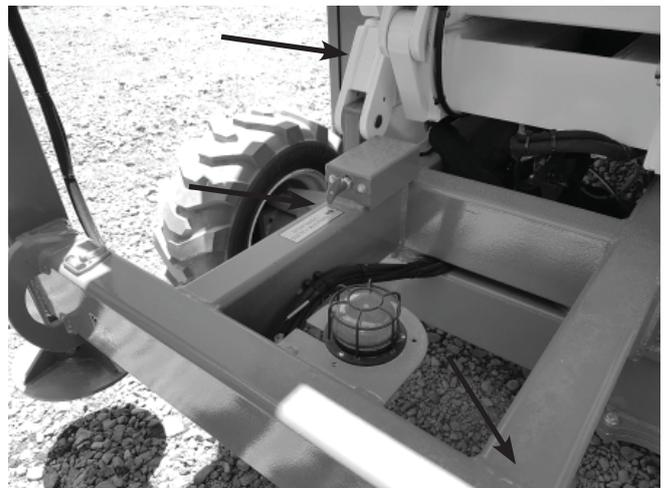
Figure 7.19 - Structural Damage and Welds
