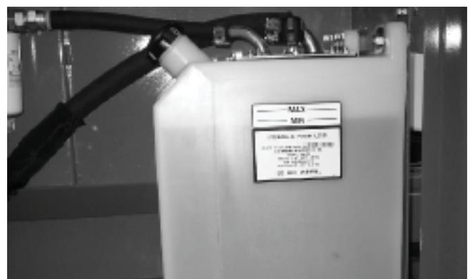
**Figure 4.4 - Hydraulic Oil Level**
