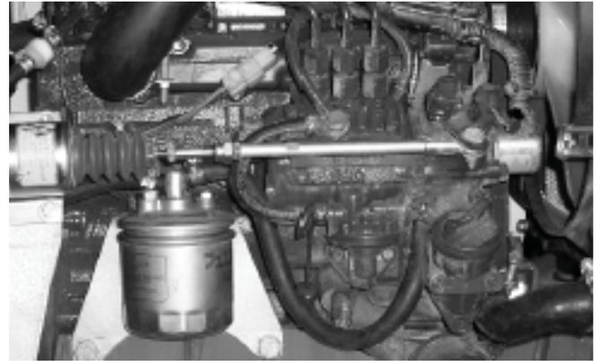
Figure 7.4 - Fuel Leaks in Hoses & Joints
