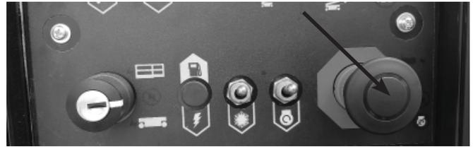
**Figure 2.2 - Ground Control Box Emergency Stop Switch**
