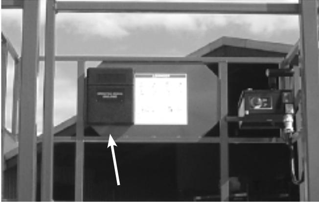
**Figure 7.32 - Operator Manual Holder**
