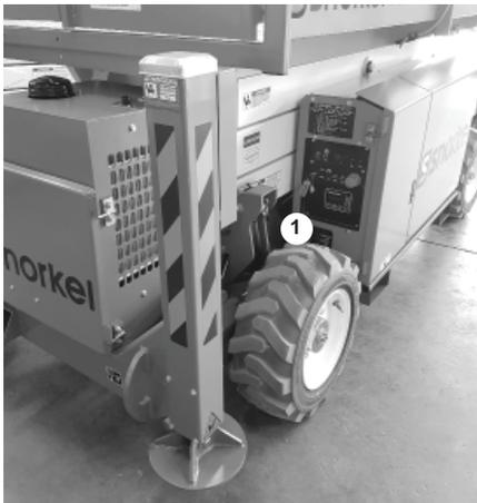
**Figure 6.1.1 - Control Box Location, Ground Position**
