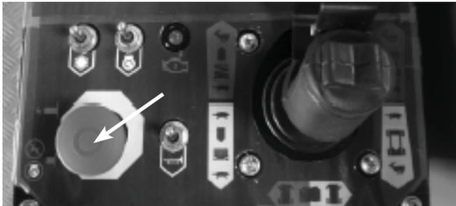
Figure 9.1 - Platform Control Box Emergency Stop Switch
