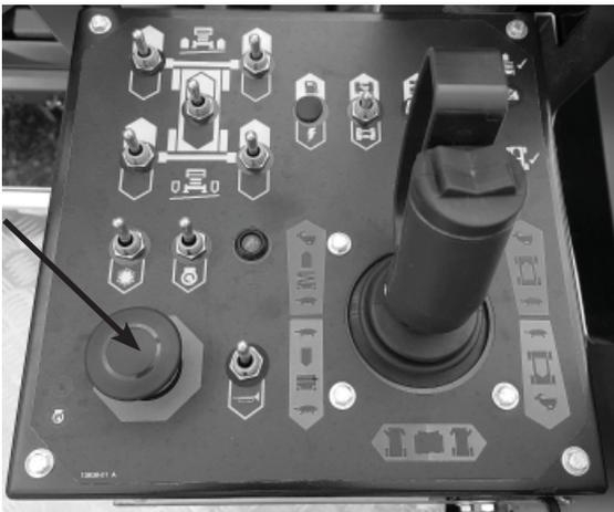
**Figure 2.1 - Platform Control Box Emergency Stop Switch**
