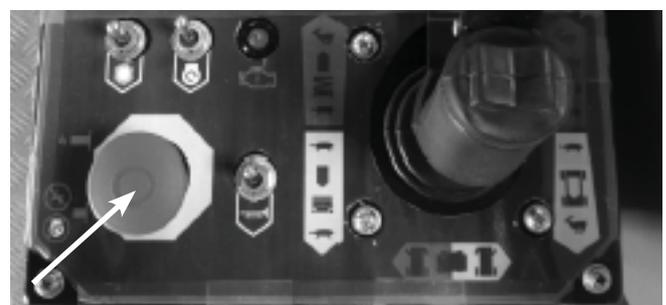
Figure 8.2 - Emergency Stop switch at Platform Control Box
