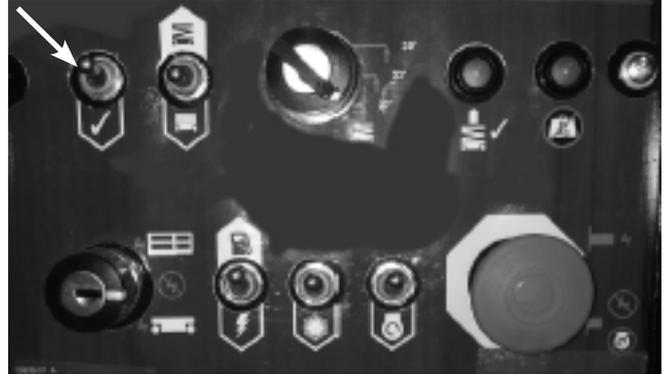
Figure 2.12 - Enable Switch
