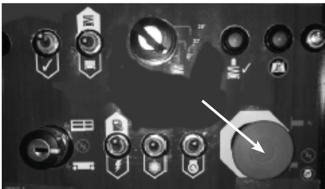
Figure 9.2 - Ground Control Box Emergency Stop Switch
