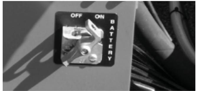
**Figure 6.2 - Battery Switch**
