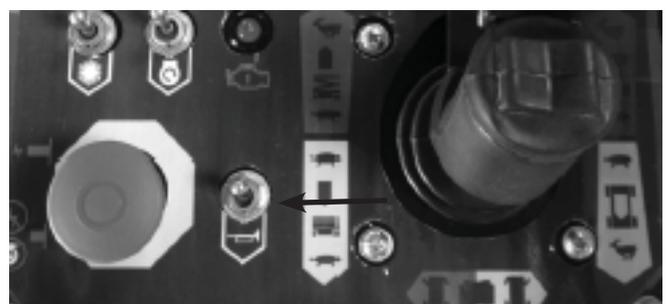
Figure 2.10 - Operator Horn
